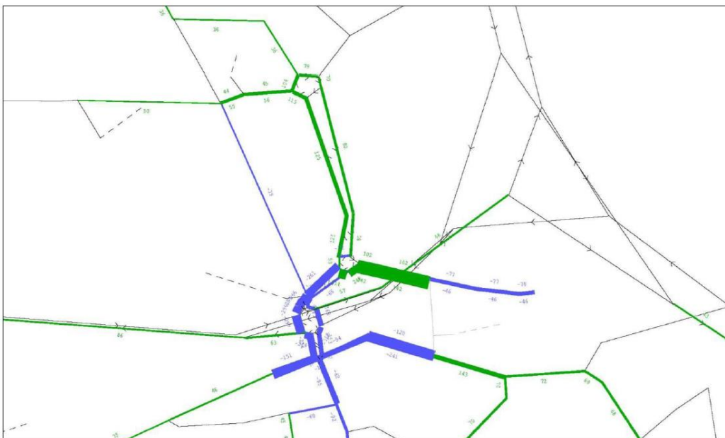
Figure 4: Traffic Flow Difference Plot With and Without Link Road Scheme – 2019 PM Peak Hour
