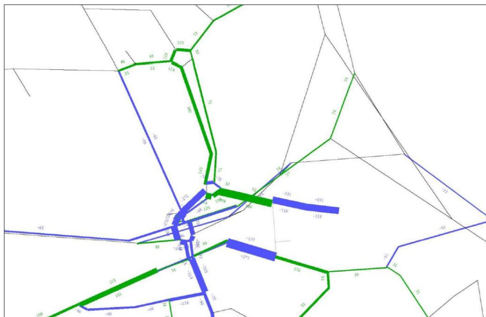
Figure 6: Traffic Flow Difference Plot With and Without Link Road Scheme - 2034 PM Peak Hour
